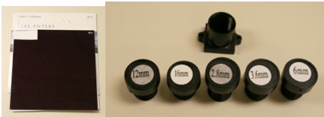
Figure 4. An IR-filter (left), a mount (top right) and different angled lenses (bottom right)
