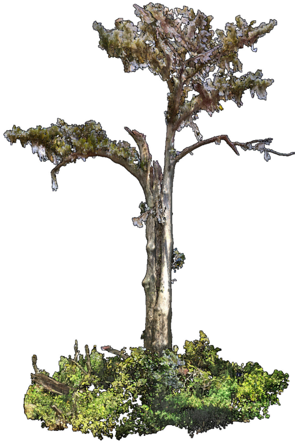
4 Point cloud of bald cypress captured with terrestrial laser scanning.
